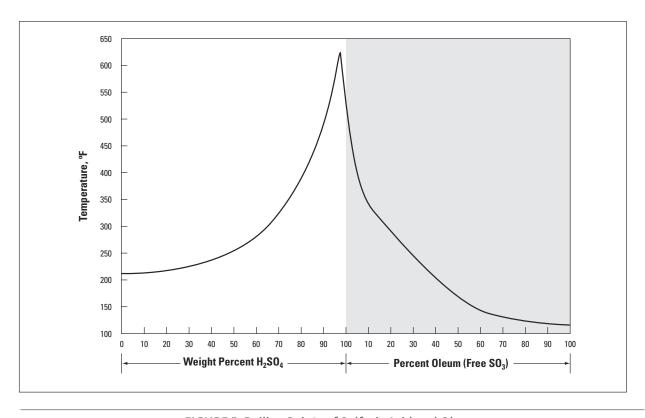
FIGURE 5: Boiling Points of Sulfuric Acid and Oleum
