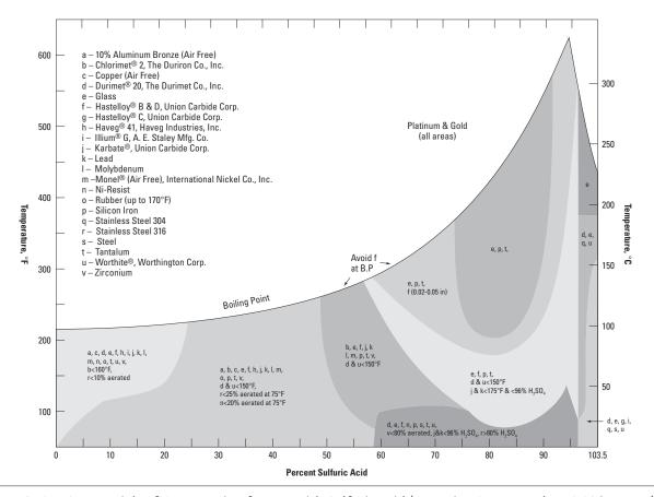
FIGURE 10: Materials of Construction for Use with Sulfuric Acid (Corrosion Rate Less than 0.02 in per yr)
