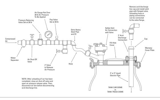
FIGURE 8: Air-Piping Arrangement for Unloading Acid Tank Cars
