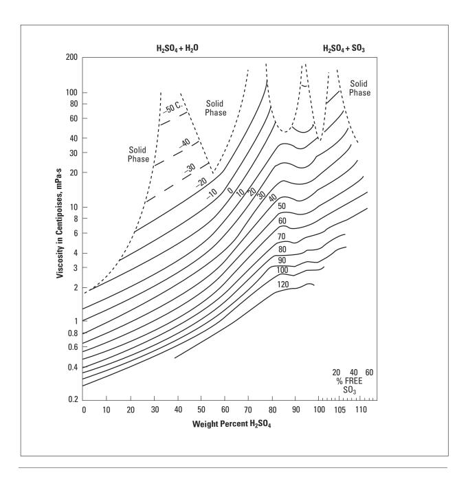
FIGURE 6: Viscosity of Sulfuric Acid Solutions
