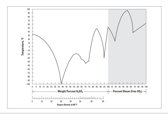
FIGURE 4: Freezing Points of Sulfuric Acid and Oleum
