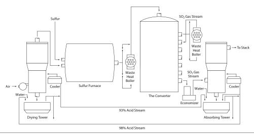
FIGURE 1: Contact Process
