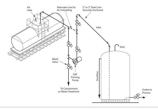
FIGURE 7: Tank Car Delivery
